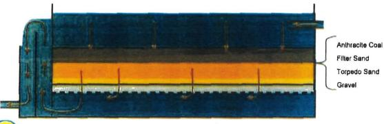
Any particles remaining in the water after coagulation and sedimentation are removed by passing the water through filters made from crushed coal. (anthracite.), send, and gravel. The filters catch the small particles and do not allow them to pass through the filter.
